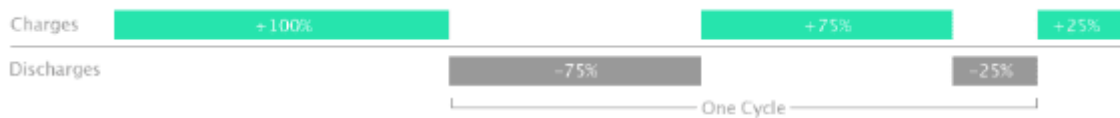
One charge cycle is completed after you've discharged 100% of your battery's capacity.
